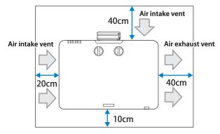
• If you are installing multiple projectors next to each other, make sure hot air from the exhaust vent does not go into the air intake vent of another projector.
