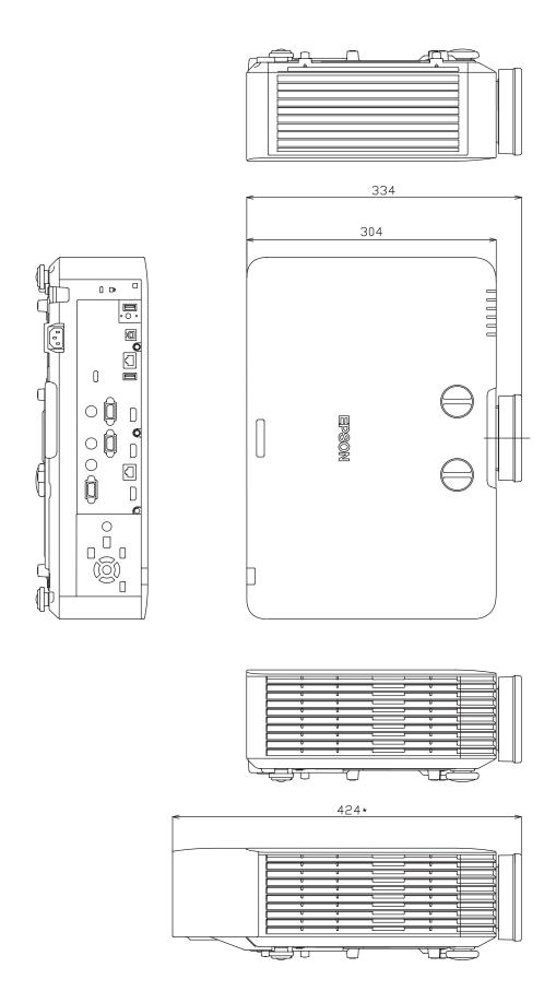
\*Dimensions when the cable cover is attached.
