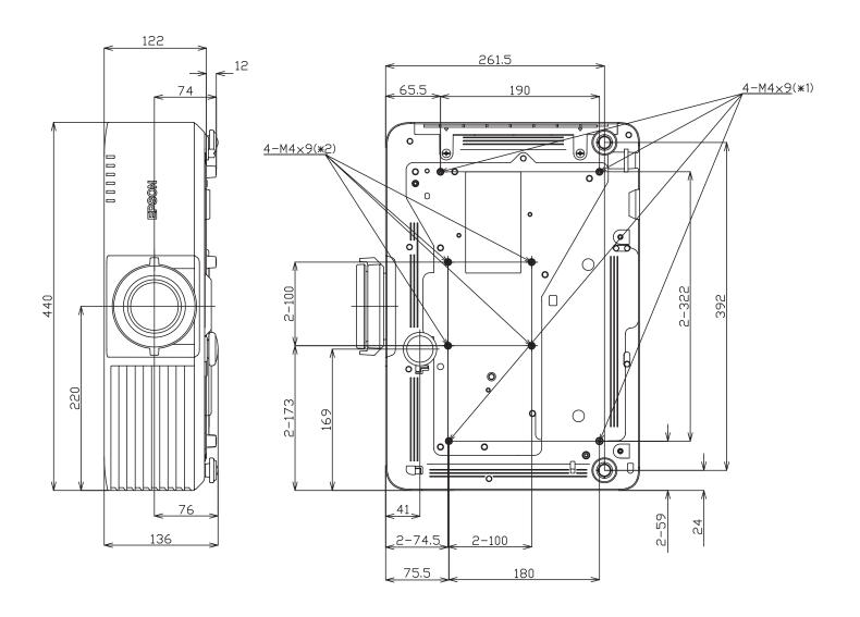
$<sup>^{\</sup>ast}1$  Mounting section for optional mount.  $^{\ast}2$  Mounting section for mount conforming to VESA standards (100 x 100 mm).
